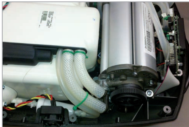
Figure 25: Installing the Compressor Intake Filter.
